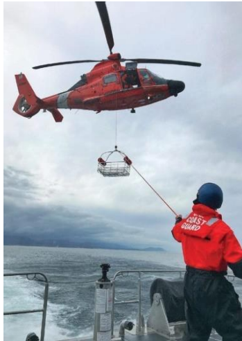
Photo Caption: an MH-65D demonstrates a ‘trail line hoist’ with a Coast Guard small boat. Note the hypotenuse or diagonal formed by the trail line running from the person on deck to the hoist hook.
